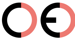
False CE Mark (too far)
